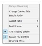
• Enable Audio: Enables audio transmission with remote locales. Select to display (Select to display)
